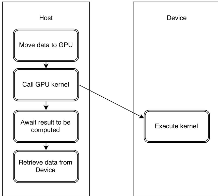
**Figure 2.1:** A typical CUDA execution flow.
